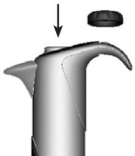
to change the filter daily (after 50 - 250 pipetting cycles) and always in case of over-aspiration. (See Chapter 2 for ordering information.)
