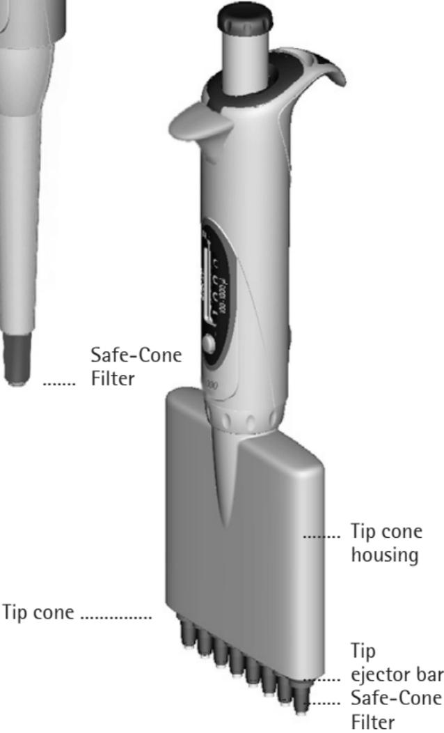
The special tip cone design of the pipette offers the possibility to use replaceable Safe-Cone Filters to help prevent the contamination and damage of the pipette. The operating button of the mLINE allows safe and easy filter ejection. The pipette uses disposable tips.
